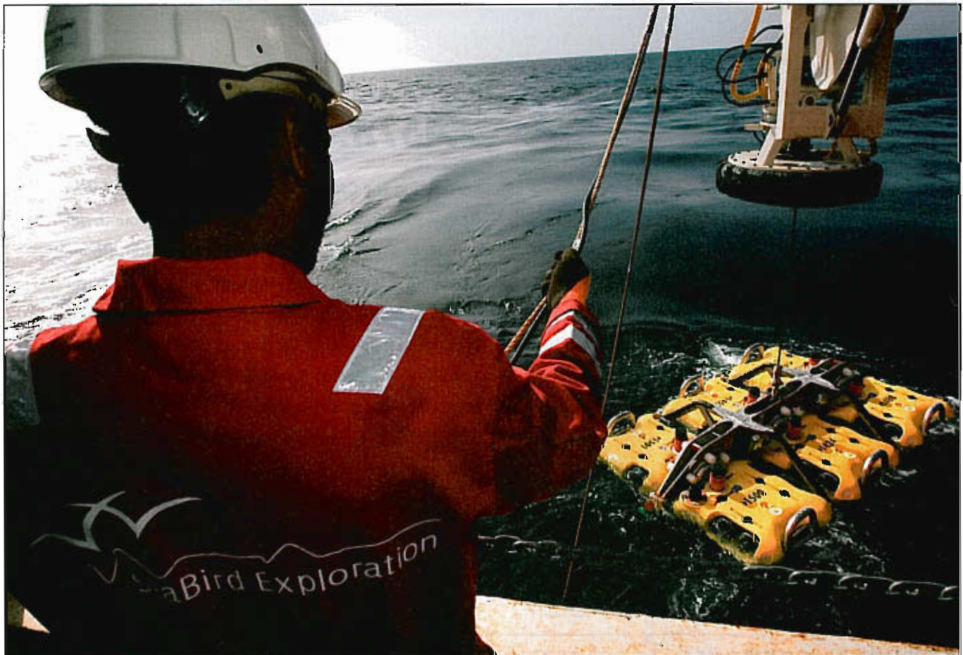
Batch of SeaBird seismic receiver nodes being lowered to the seabed for placement by ROV.
