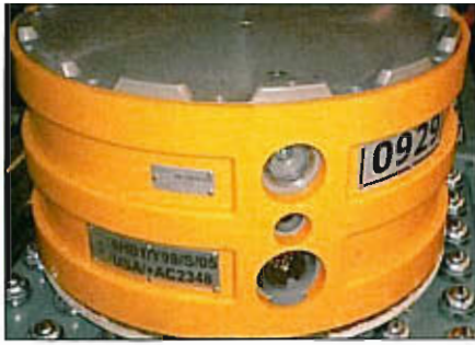
LEFT: Business end – Z3000 node containing three geophones and a hydrophone.
